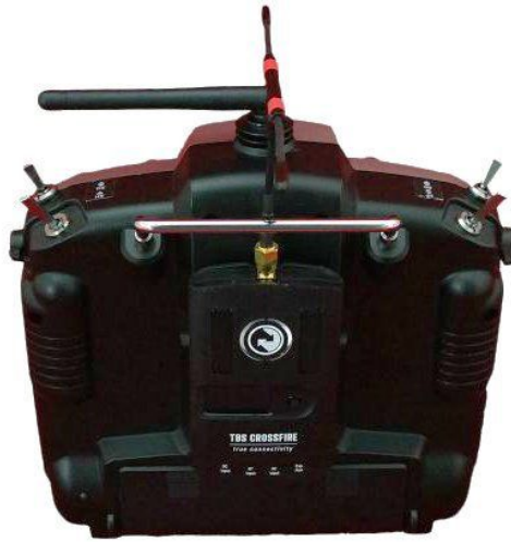
Correct transmitter antenna mounting direction
