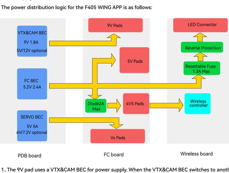
1. The 9V pad uses a VTX&CAM BEC for power supply. When the VTX&CAM BEC switches to another voltage through the pad jumper, the 9V pad will output the corresponding voltage.
