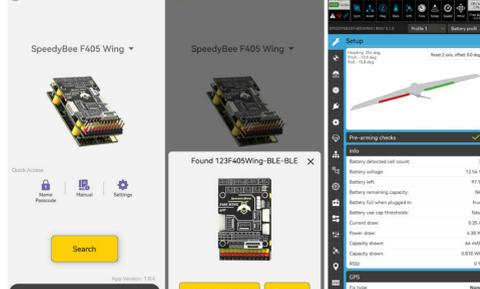
● Suitable for different flight control firmware and Configurator. The supported apps are listed in the following table. It is recommended to use Bluetooth BLE mode for iNav and WiFi mode for Ardupilot.
