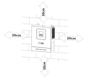
Install the unit by screwing three screws. It's recommended to use M4 or M5 screws.
