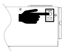
Once the unit has been properly installed and the batteries are connected well, simply press On/Off switch (located on the button of the case) to turn on the unit.
