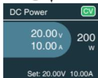
On the main menu, hold the ENTER button for two seconds to enter System Setting>DC Power.
