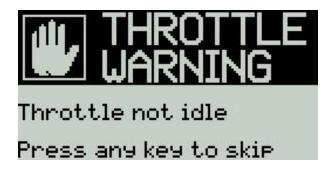
**Switch warning:** This is a warning that a switch on the radio -control is not in the default position. (The default setting is that all switch directions are up 1)
