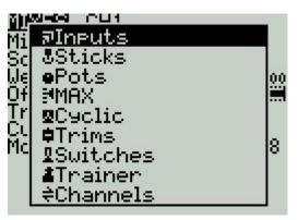
Weight: Channel travel amount, the range is -500 / + 500. The default value is 100. Negative values indicate reverse channel output.
