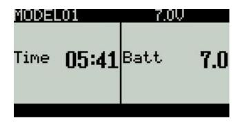
By pressing TELE from the main interface, vital telemetry information can be quickly displayed. Radiomaster has set two values- Time and Batt (system battery voltage) as defaults; these values can be changed by the user- displaying up to 4 values
