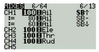
To edit a mixing control, use the scroll wheel to select the mixing control item up and down, and press and hold the ENT key to enter the editing submenu. Select Edit and press the ENT key momentarily.
