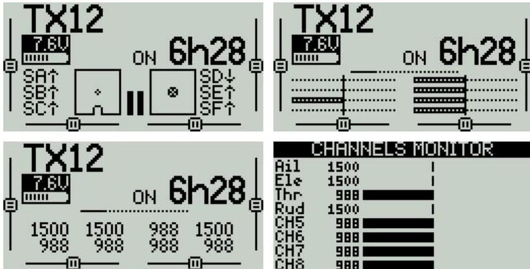
The main interface can display the following information: Model name, TX voltage, gimbal/switch position and trim location.
