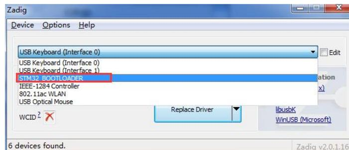
D. Click the Replace Driver button (if the driver has been installed before, Reinstall Driver will be displayed) to replace / install the driver. After the driver installation is completed, you can use OpenTX Companion to write the firmware to the radio controller correctly.
