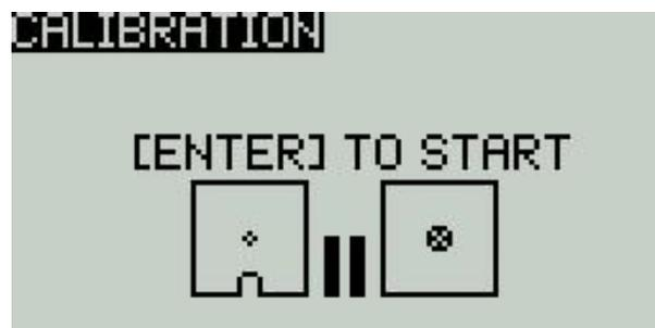
C. In the second step, place all the gimbals, knobs, and side sliders in the middle position. The system obtains the midpoint value, and then press the confirmation key to continue to the next step.
