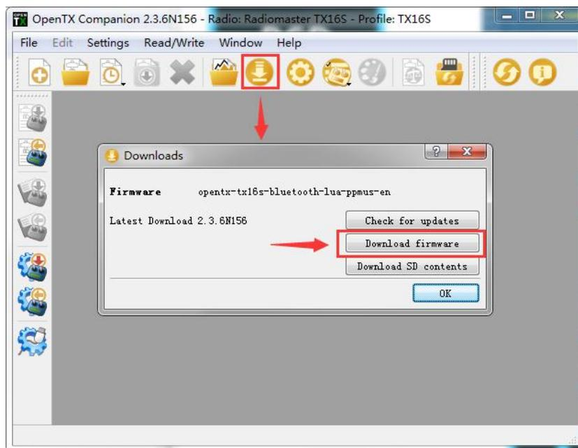
Before writing the firmware, please make sure that the radio control is turned off, and plug in the supplied USB-C (TYPE-C) cable. The following device name will appear in the computer device manager:
