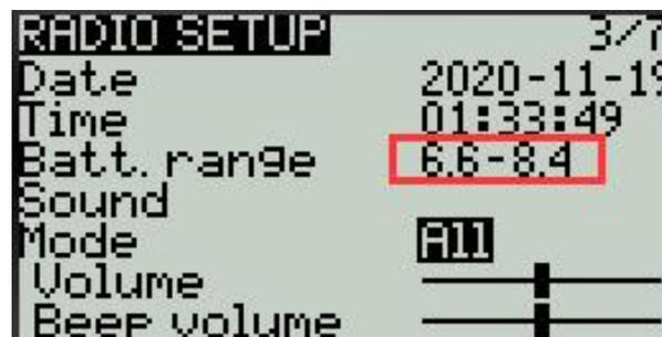
C. On the current page, turn the scroll wheel to find Battery low (low voltage alarm), and fill in the alarm voltage as shown below. When the radio-control voltage is lower than the current set voltage, the system will play a voice alert and report that the battery voltage is low.
