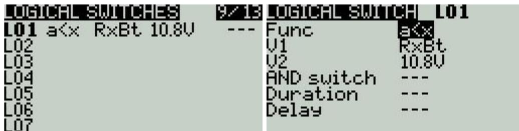
The setting of the L01 example in the figure is expressed as follows: When the return value V1 is less than 11.0V, the L01 switch is automatically turned on. In the settings of other pages, L01 has the same function as the physical switch. You can define the corresponding function for L01 on or off. In this way, a switch is automatically executed according to the parameters that change in real time.
