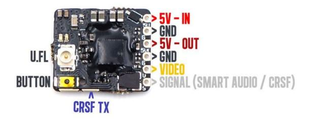
The UNIFY PRO32 5G8 nano comes with pre installed silicon wires for easy installation in your build. There is a filtered 5V input with a 5V output for your camera.
