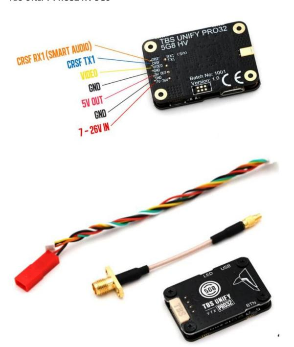
The UNIFY PRO32 5G8 HV comes with a cable assembly with silicon wires for easy installation in your build. There is a filtered 5V output for your camera.
