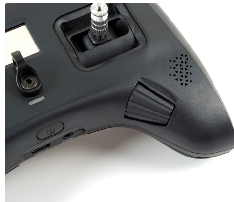
Rocker switch, power button, ports and speaker
