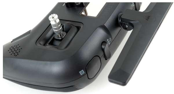
Rocker switch, power button, ports and speaker
