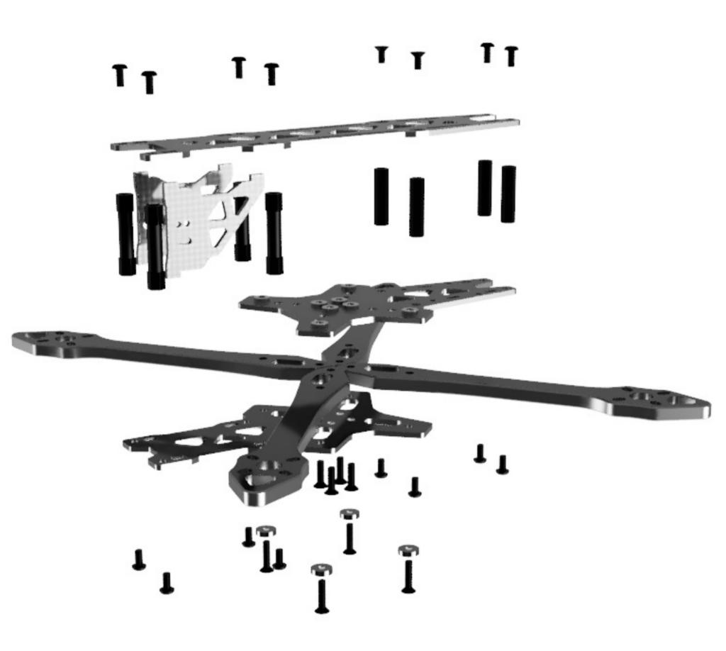
Insert  $12\,\text{mm}$  countersunk screws on the edges of the bottom plate
