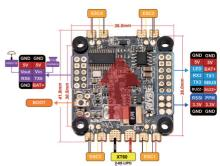
ESC M1-M4: For esc power cable
