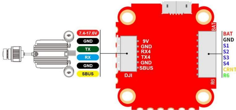
3.5.8G VTX serial port opens. The protocol is selected according to its own VTX protocol.
