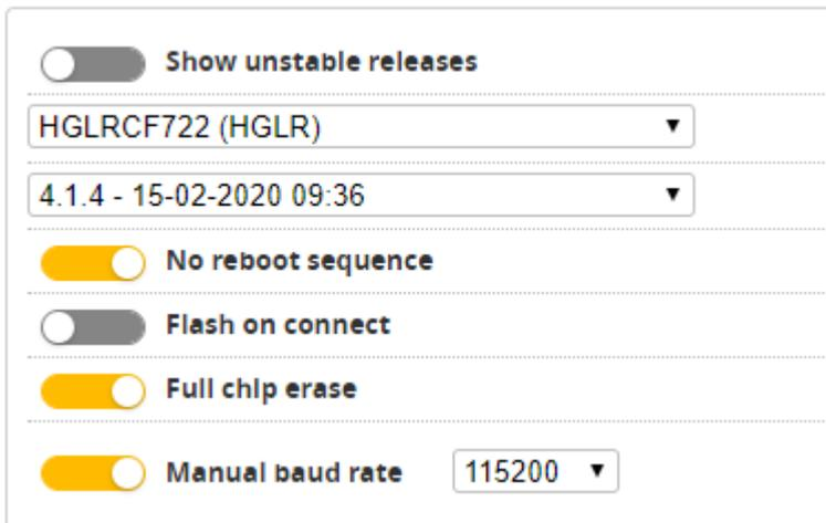
6. Click **Load Firmware [Online]** Load firmware. **Flash Firmware** Waiting for completion **Erasing ...** It will be prompted upon completion.
