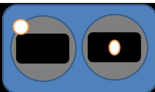
The graphics above show the stick command to bring up the OSD menu. The stick command is: throttle centered, yaw left, pitch forward. The exact stick command therefore depends on which mode your transmitter sticks are in.
