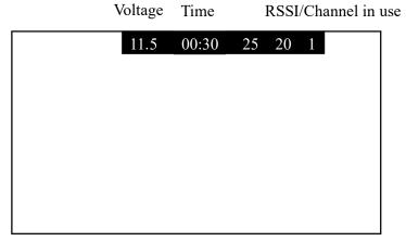
**Voltage indicator:** input voltage value is displayed; Display from 10V to 26 V. When the battery is low, the menu turns red and starts flashing. When the battery is too low, the blue light flashes faster and faster in the lower left corner and the buzzer alarms. Please replace the battery immediately to avoid damage to the battery.
