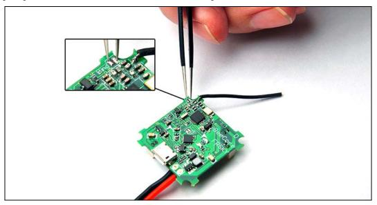
b)Turn on your Radio and select D8 mode for the Receiver. Then Go to the Receiver [Bind] option, and ENT to Binding with the BEECORE. The LED Combo (2 Red and 2 White) will turning off and then get to be solid if binding successfully. Reconnect the battery to the BEECORE after Binding successfully.
