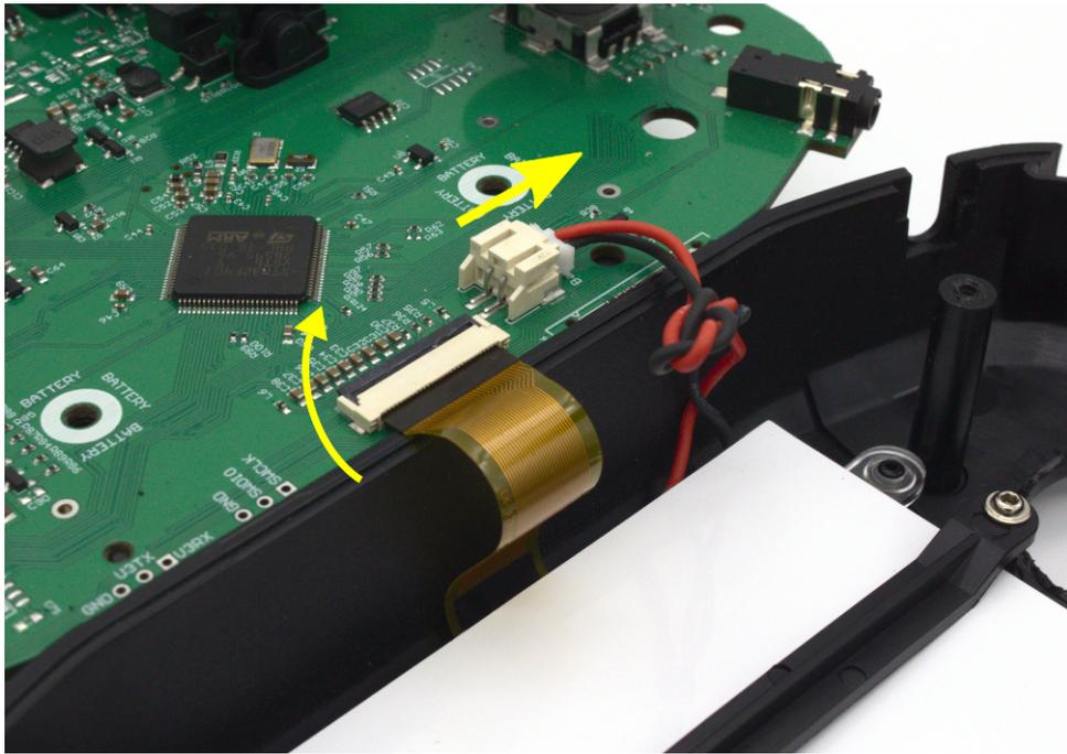
The gimbal support pegs are inserted on the mainboard holes and easily pulled out. Insert the new gimbal(s) and re-assemble the radio. Flap the PCB over the front shell, slide the switches into their holes, place the trim switches with a tweezer and gently push it in. Install the screws holding the PCB. Gently tighten the switch nuts down and not overtighten them!
