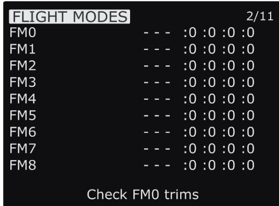
Create flight presets that can activate a particular attitude or characteristics of the model
