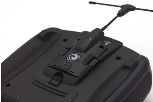
JR bay with installed TBS CROSSFIRE module
