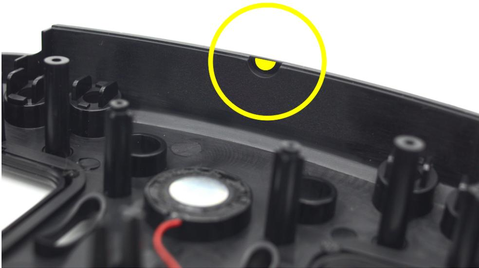
Feed the antenna wire around the internal PCB antenna and place the new SMA connector with the included washers in the hole, re-assemble the radio and tighten the nut down.
