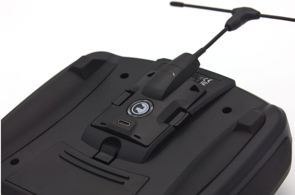
Now enable the external module in the model settings and select the correct protocol type for your module. For the TBS CROSSFIRE, you need to use it to CRSF.
