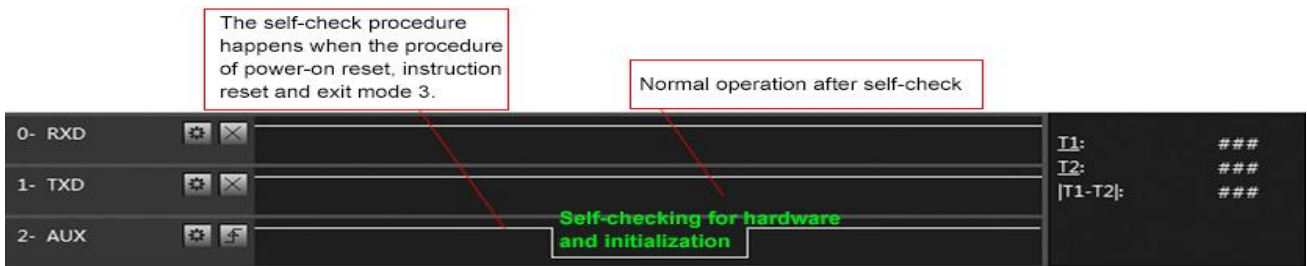
Timing Sequence Diagram of AUX when self-check
