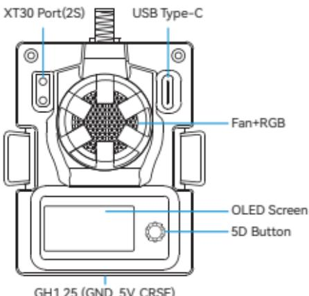
**Note: Please DO NOT use 3S or above battery to power up the TX module. Otherwise, the power supply chip in the TX module will be damaged permanently.**
