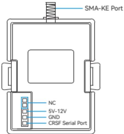
**Note:** Please assemble the antenna before power on. Otherwise, the PA chip in the RF TX module will be damaged permanently.
