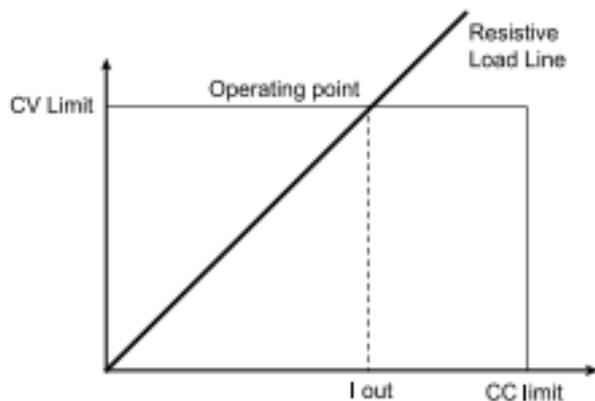
Power Supply I-V Diagram, CC Operation
