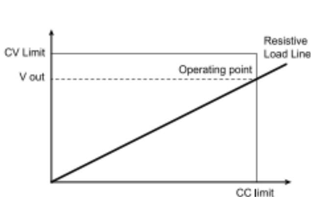
Power Supply I-V Diagram, CV Operation
