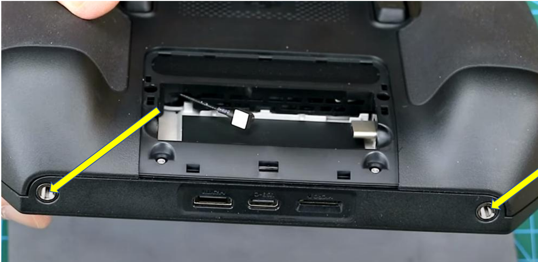
Step 4 remove the two hidden screws. Pry open this remote control along the edge
