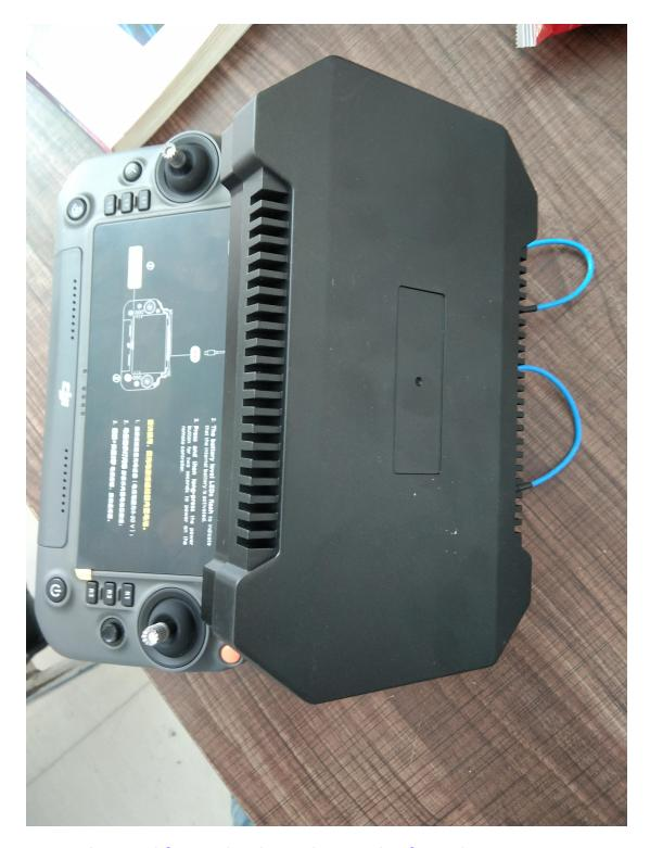
Insert the amplifier and tighten the circular fixing button to secure it.
